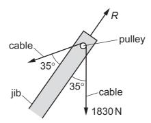
The force *R* that the pulley exerts on the cable is in line with the jib. The cable and the pulley are in equilibrium.
