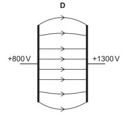
**31** The diagram shows two metal plates P and Q. There is a potential difference of 700V between the plates. Plate Q is earthed.
